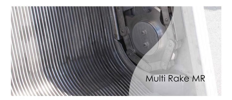
Multi Rake MR is a modern mechanically raked coarse bar screen that separates debris and rubbish from influent.
