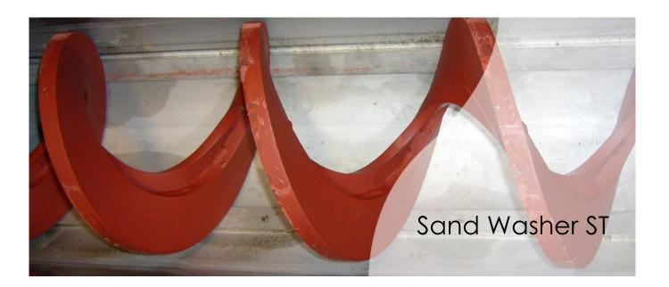
Sand Washer ST separates, washes & dewaters sand from water. Street sand, filter sand and similar materials can be handled.
