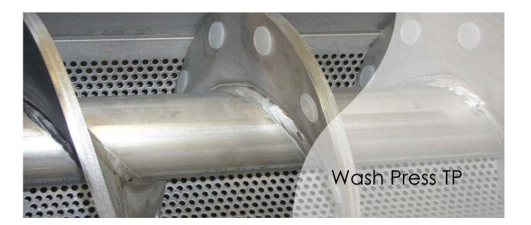
Wash Press TP is a screw press for washing, compaction and conveying of screenings and wet waste.
